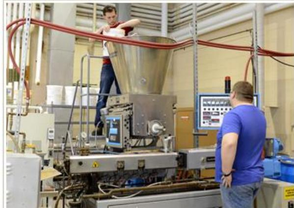
Members from David Grewell's research team extrude soy flour and PLA using CCUR's pilot-scale extruder. Matt Blom, a student in industrial technology, (right) sets the extruder's controls as James Burkholder, a student in materials engineering, feeds the soy-PLA mixture into the hopper. [Larger image](#)
