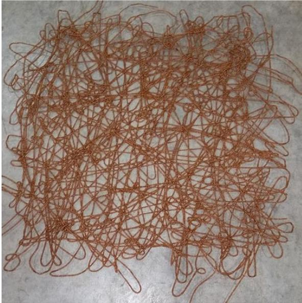
Figure 5- PHA/DDGS ECP sheet at 60/40 formulation.
