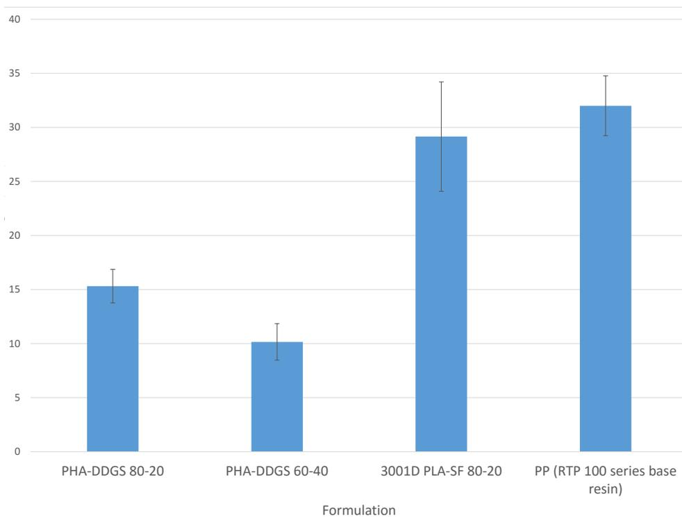
Figure 7. Tensile strength of three corn-based resins compared to petrochemical plastic (PP)
