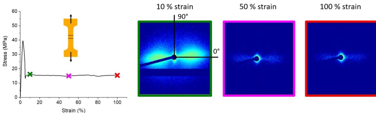
Figure 1. The left image is a tensile stress-strain curve of “tough” neat PLA (aged < 2 hrs.), where the different X symbols correspond to the strain at which the tests were terminated and the material was subsequently analyzed by SAXS. The right images are 2-D SAXS patterns at specified strains, where the samples were stretched in the vertical direction.
