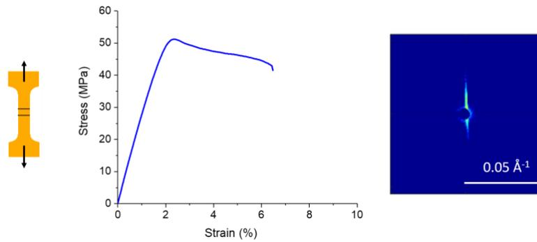
Figure 2. The left image is a tensile stress-strain curve of “brittle” neat PLA (aged > 2 days). The right image is a 2-D SAXS pattern, where the sample was stretched in the vertical direction until failure.
