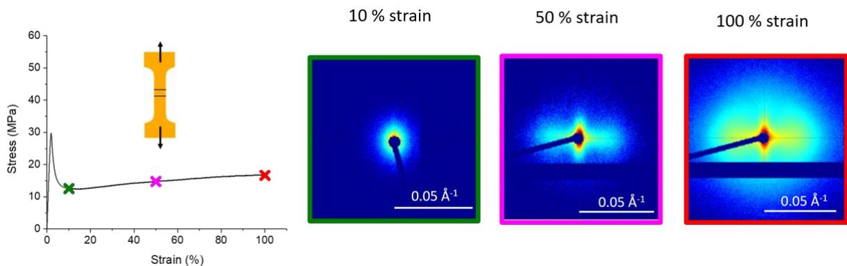
Figure 3. The left image is a tensile stress-strain curve of PLA/PBO-PBO blend (aged for 2 days), the different X symbols correspond to the strain at which the tests were terminated and the material was subsequently analyzed by SAXS. The right images are 2-D SAXS patterns at specified strains, where the samples were stretched in the vertical direction.
