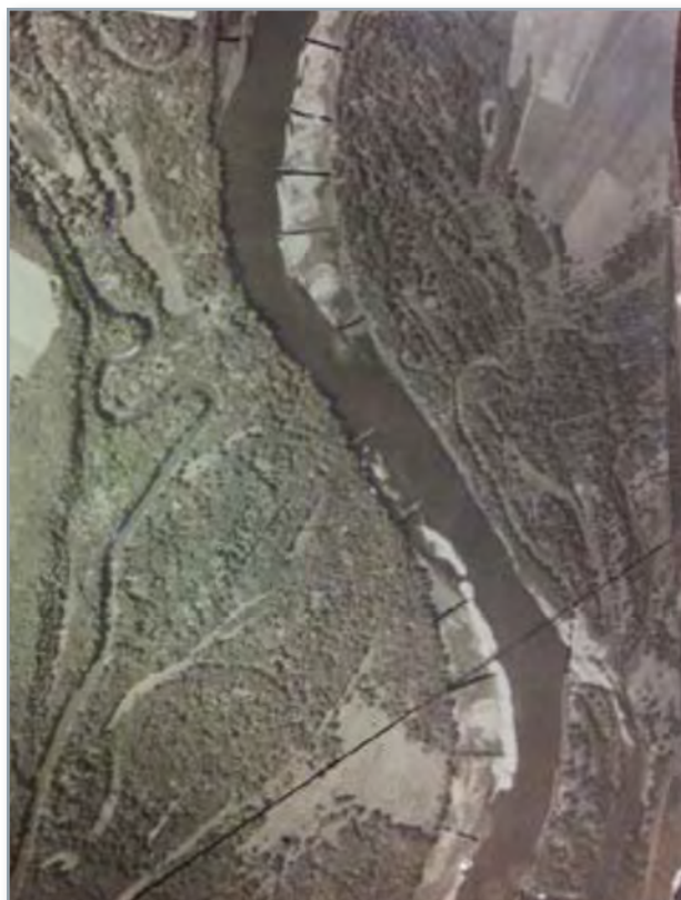
Figure 1. An example of series of wing dams (small black lines) along the Upper Mississippi River (From Army Corps of Engineers). The PIs have gathered series of these maps showing the location of wing dams in the upper Mississippi River.
