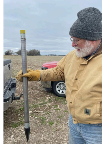
Figure 1.2b – Bottom tip of the galvanized pipe installed during the Spring and Summer 2021 with two additional in fall 2023.
