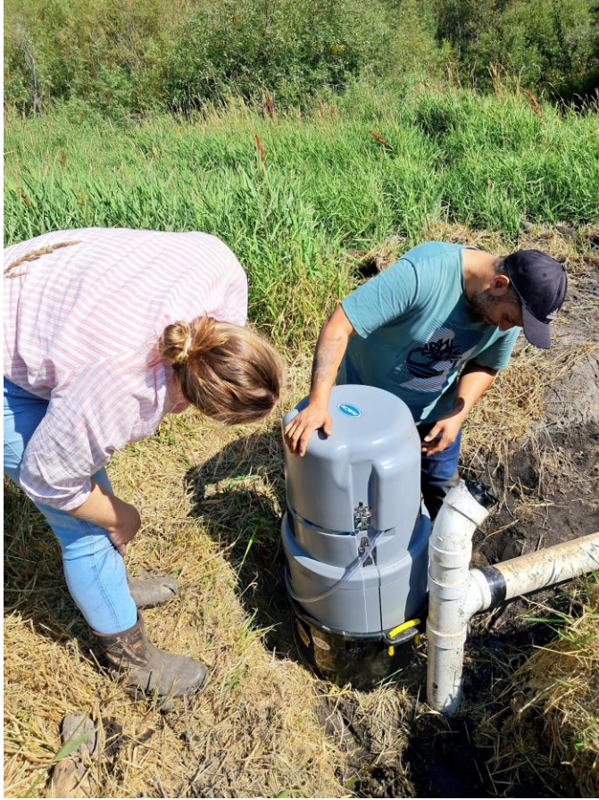
Dr. Lindsay Pease (right) and Dr. Murad Ellafi (left) of University of Minnesota installing an automated water sampler at the bioreactor outlet in August 2024.
