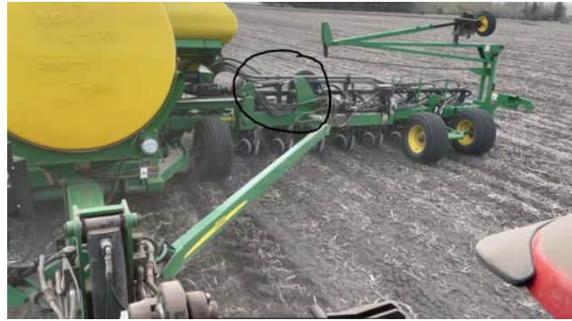
Figure 2: Planting corn in the trial plot. Circle shows the weight distribution system installed on the planter.
