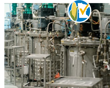
Valerian used 300-liter fermentation tanks (shown above) to produce its proprietary monomer as part of a Minnesota Corn-supported project.
